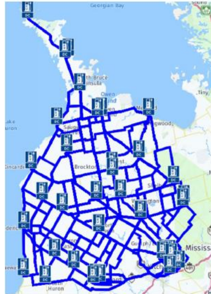
Figure 2: Regional EV charging network (including existing stations) after installation of recommended Level 3 EV charging stations. Blue lines indicate which routes are travelable by an EV without any range limitations.
